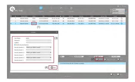
5. After activation, you can change the IP address or other network values, and then click "Modify" button to change the IP address successfully;
