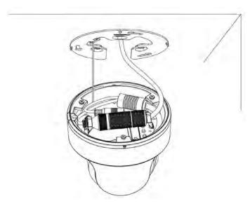
Step2: Rotate the camera to bracket and tighten the setscrew;
