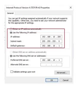
B. Click "Advanced", and then click "IP settings" > "IP address" > "Add". In the pop-up window, enter an IP address that is in the same segment with your Avycon IP camera (e.g. 192.168.10.200, but please confirm that the IP address you pick does not conflict with another address on the network);
