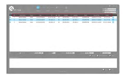
3. Select a camera or multiple cameras according to the MAC addresses; the camera must be assigned an IP address to be accessible.
